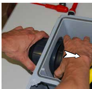
18. Unlock the exhaust spigot.
