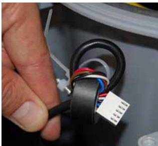
23. ...and replace it by following the same scheme. Note: The wire must be passed through the tore 2 turns!
