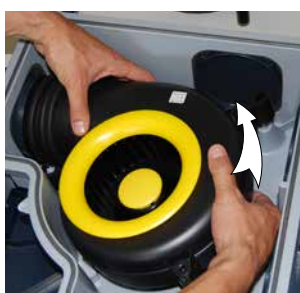
19. Withdraw the mototurbine.
