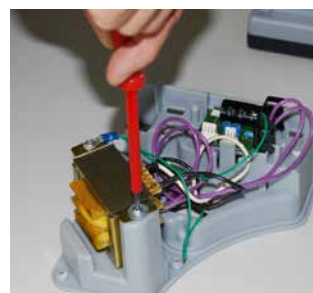
7. Unscrew the supply (2 screws).
