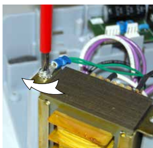
14. Fix the supply (2 screws) Warning: Tooth-pressure must be in contact with the supply!
