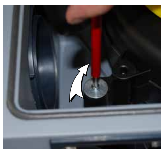
25. Fix the mototurbine (3 screws).
