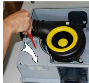
29. Fix the trap door (1 screw)
