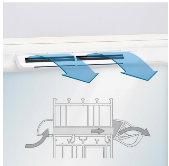
Figure 4: EMM 2 window inlet
